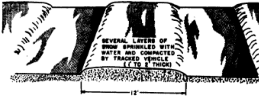
Figure 5-7. Road reinforced with snow.
